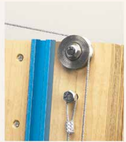
Cable Hook. The cable is attached to the saw base with a hook made from a piece of aluminum angle.
