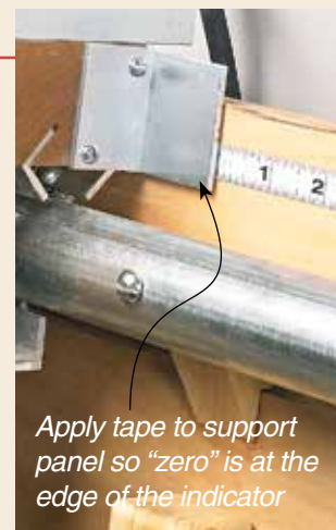
MEASURING TAPES. Finally, in the box below, you can see how I added a pair of measuring tapes to set up for accurate cuts.
